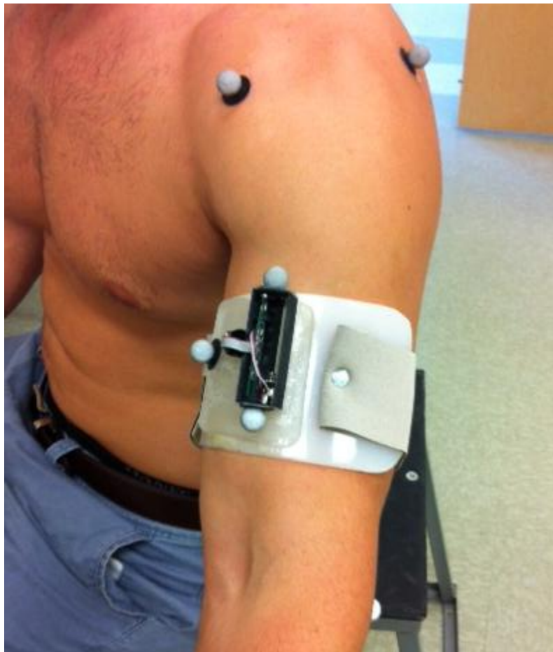
Figure 26: The sensor cuff and Slip Detection Sensor being used to compare the sensor's output to the motion analysis system data.
