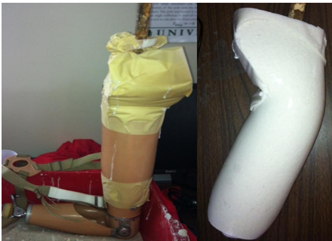
Figure 28: Process for making the positive mold representing the internal socket shape.
