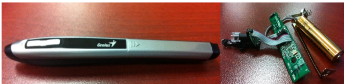
Figure 20: Left: Pen mouse; Right: Sensor and circuit board.
