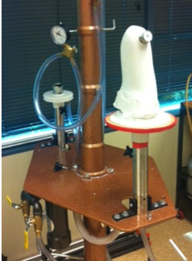
Figure 29: Plaster mold with a suction valve is placed upside down on the vacuum rig.
