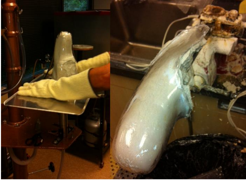
Figure 32: Forming the thermoplastic over the plaster mold, and removal of the excess material.
