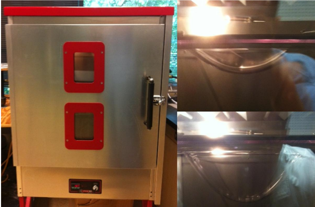
Figure 31: Oven used to heat the thermoplastic and drooping of the thermoplastic at two different time periods. The thermoplastic forms a blister, hence the name of the technique.
